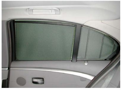
When the window is open and a command to raise the side-window roller blind is sent, the side-window roller blind starts up briefly and reverses. This indicates that an invalid operation has been attempted. The roller sun blind cannot be raised until the customer closes the window. It is always possible to operate the quarter roller blind, irrespective of the side window position.
